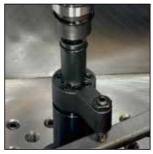
Note: The clamp arm can be replaced with a custom one of your own design. Refer to the instruction on our website for the dimensions and details. Note that the clamping force with the custom clamp arm may increase or decrease from the values above.
