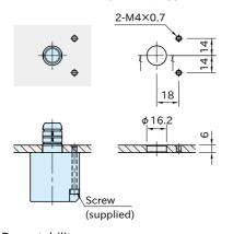
With M5 Low-Head Cap Screws (customer supplied) (Dimension: head dia. 8.5, head height 3.5)
