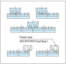
Can attach various fixed jaws at different positions on the base.
