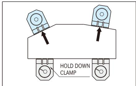
For clamping of an initial workpiece, tighten the clamp temporarily and Hold Down Stops (Swivel Stops) at a prescribed position. After that, tighten the clamp finally.
