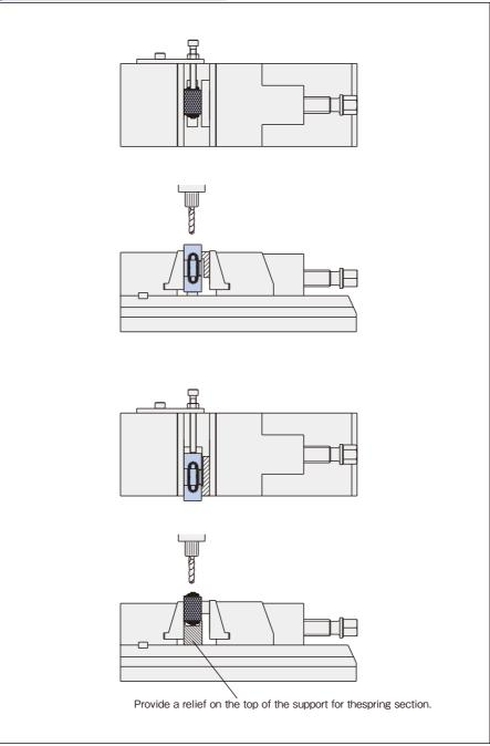
Jaws may be machined in disassembly.
